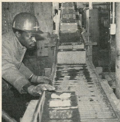
Left: Block plant has BECO ABC system for moving units in and out of kilns. Right: Cured block head for cubing station under watchful eye of worker.
